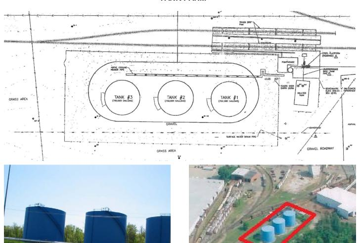
Tank Capacity: 3 Steel Tanks of 750,000 gal. each (2.2 million gal. total)
